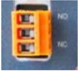
NO = Normal open contact, is open in alarm condition
